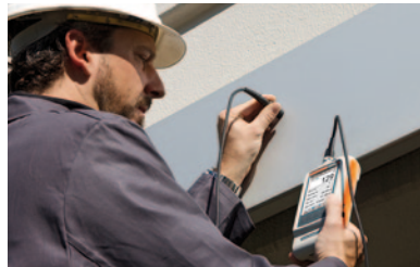
Measurements of anodised aluminum on a façade
